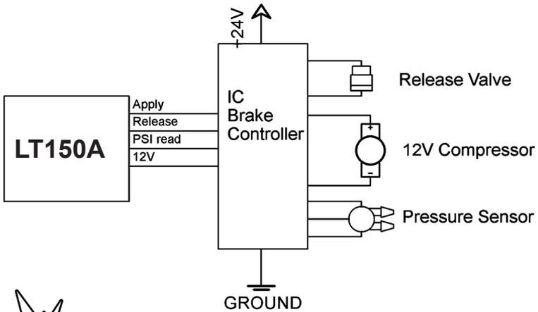
**!** The Pressure sensor shown in this diagrams is actually inside the Brake Controllers. It does not have to be connected up electrically.
