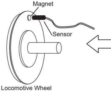
The LT150A needs a pulse signal to ground on its speed input connection to measure speed.
