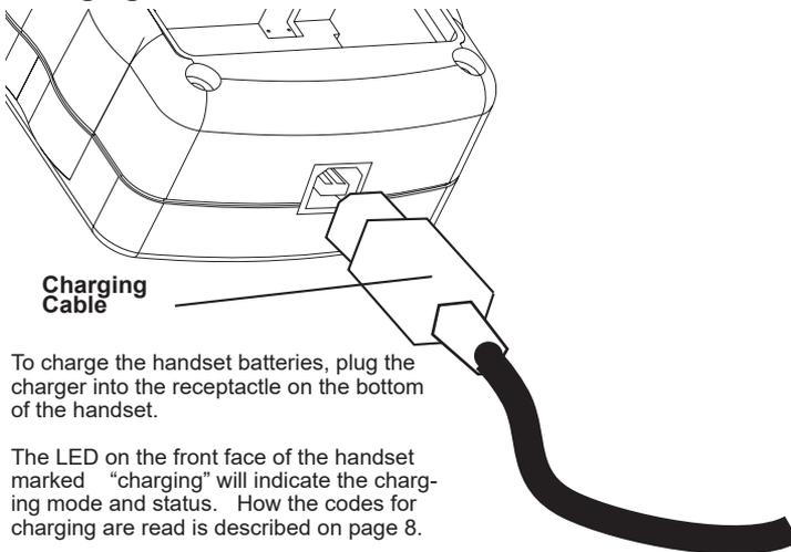
To charge the handset batteries, plug the charger into the receptacle on the bottom of the handset.
