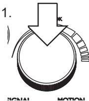
1. Press the knob while not in brake-lock mode. The display switches from showing the regular dash to a screen showing the voltages of the locomotive batteries.
