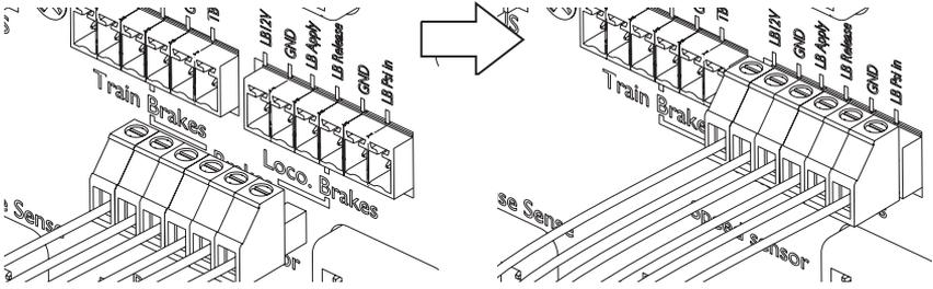
Plug the 6 pin brake phoenix connector into the Loco brake receptacle.
