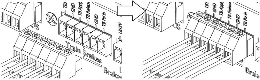
Plug the 6 pin brake phoenix connector into the Loco brake receptacle.
