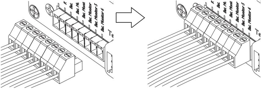
Plug the 8 pin Phoenix plug into the system monitor receptacle
