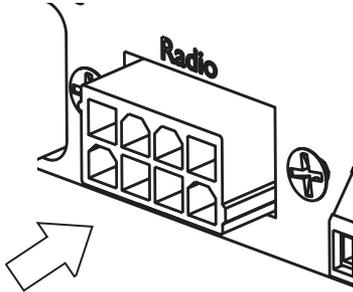
Plug the radio transceiver into the 8 pin receptacle on the frontpanel of the LT150A controller
